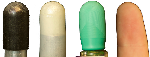
Fig. 2. Size and shape of artificial fingers alongside the human finger used for comparison. Shown from left to right are the TangoPlus, Dragon Skin, BioTac, and human fingers.
