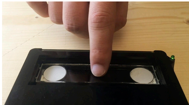
Movie S1. Effect of the modulation of friction on the finger dynamic during exploration. The green LED on the right indicates that the ultrasonic vibration is turned on. The high-amplitude vibration creates a drastic reduction of the coefficient of friction that facilitates finger motion.
